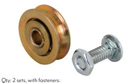
Steel ball bearing roller, 1 in. O.D., 1/4 in. I.D. axle hole, center grooved, steel carriage bolt and nut.
