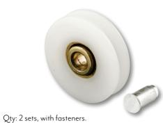
Plastic ball bearing roller, 1 in. O.D., 3/16 in. I.D. axle hole, center grooved, aluminum rivet.
