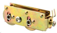
Steel housing assembly, end adjustable, 1-1/8 in. O.D. tandem steel ball bearing rollers, center grooved.
