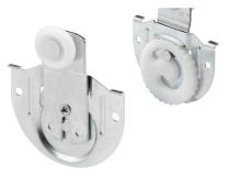
Steel bracket, plastic adjusting wheel, top hung, adjustable, 7/8 in. O.D. plastic roller, round edge, for 3/4 in. to 1-3/8 in. thick doors.
