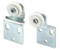
Steel bracket, 3/8 in. and 1/2 in. offset, top hung, adjustable, 3/4 in. O.D. plastic ball bearing roller, round edge, for 3/4 in. to 1-3/8 in. thick doors.
