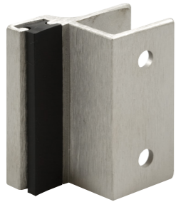
Qty: 1, with fasteners. Outswing for slide latch, for square edge posts, 1-1/2 in. hole spacing. 656-9375 (Chrome plated zamak – for 1 in. thick posts) 656-6488 (Chrome plated zamak – for 1-1/4 in. thick posts) 658-9910 (Satin cast stainless steel – for 3/4 in. thick posts, no fasteners ) 656-9909 (Satin cast stainless steel – for 1 in. thick posts)
