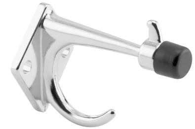
Qty: 1, with fasteners. Rubber bumper, 1-1/8 in. hole spacing, 3 in. projection. 656-7214 (Chrome plated zamak) 656-7214-T (Chrome plated zamak, with T-27 fasteners )
