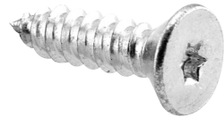
Qty: 100 T-20 flat head, six lobe with center pin, #10 x 1 in. 645-0140 (Chrome) 642-0140 (Stainless steel)
